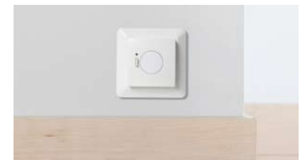
Danfoss Link™ FT (Floor Thermostat) is a relay switching on and off the heating mats/cables placed underneath the floor. It communicates wirelessly with both Danfoss Link™ CC and Danfoss Link™ RS. Simply place the Danfoss Link™ FT discreetly above the baseboard, e.g. behind curtains or drapes. Danfoss Link™ FT fits perfectly in your frame system (ELKO, ELJO and JUSSI) and is therefore easily replaceable with your existing thermostat.
